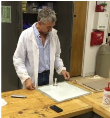
Figure 1 James Francisco prepare a vacuum bag lay up for a composite test kit sample
